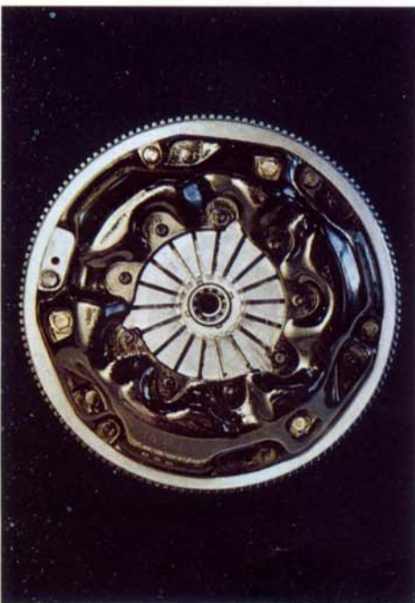
The diaphragm clutch requires less pedal pressure
